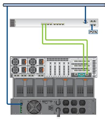
After the physical installation is completed and the cabinet is powered on you will have to follow the installation guide to configure the IP address of your ACS. You also need to configure the serial port connected to your VRTX chassis with the correct settings (115200, 8n1).
